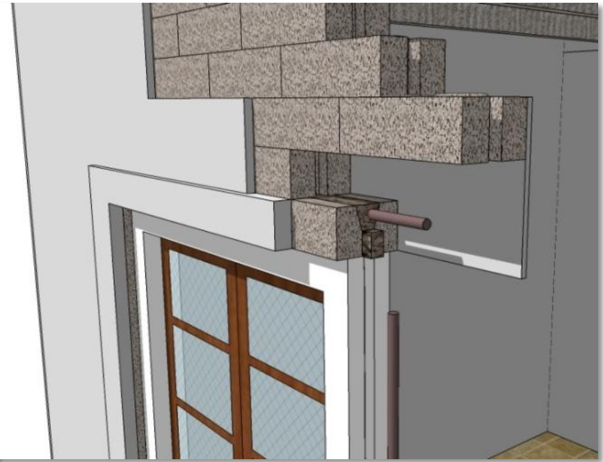
Lintel level Detail
